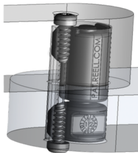
Figure 3: Installation with fastener access hole
