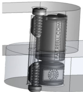
Figure 3: Installation with fastener access hole
