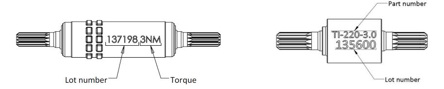
Additionally, the TI-240 is marked with the lot number and the nominal torque of the insert in N-m. The catalog number can be found by appending the torque to the TI-240 prefix. In the example shown the catalog number would be TI-240-3.0. The TI-220 is marked with the lot number and catalog number. The nominal torque is specified by the last two digits of the catalog number. In the example shown the last two numbers are 3.0, which indicates a nominal torque of 3.0 N-m.
