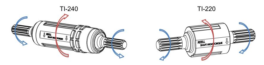
TI-200 Series parts feature text on the zinc sleeve to show the direction they apply 100% of their torque. With the parts positioned as shown, the marking on the part and blue arrows indicate the direction of high torque if the housing is held in place and the shaft is moved. The red arrow indicates the direction of high torque if the shaft is held in place and the housing moved.
