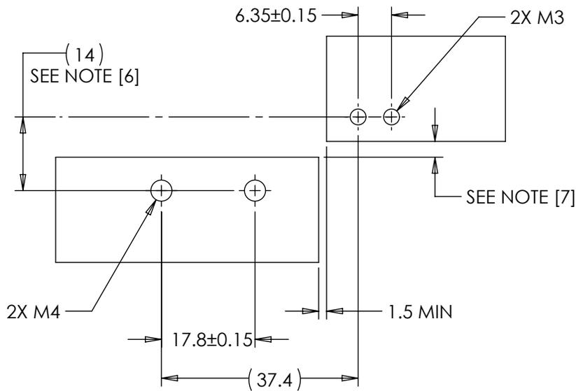
MOUNTING CONFIGURATION FOR ALL DUAL CONFIGURATIONS
