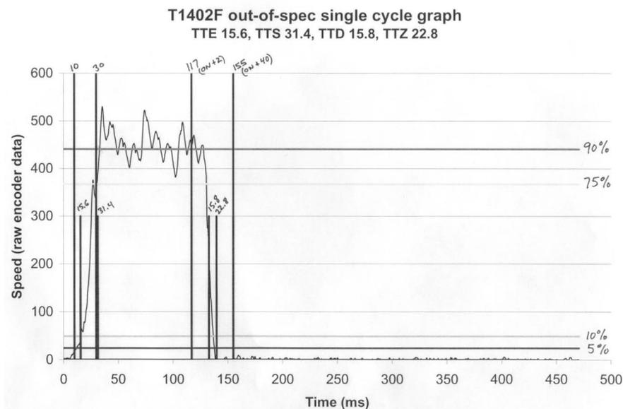
This detailed information on outlier cycles can be used for engineering design reaction. It can also be integrated to determine the position error caused by the timing shift. An example of the benefit is evaluating high TTS cycles: if the timing slip were to happen at 80% of full speed, the position error would be only 20% of that calculated by typical time-position clutch calculations.
